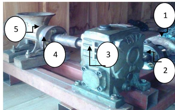
Figure 2. Pellet machine, (1) electric motor, (2) input coupling, (3) gearbox, (4) output coupling, (5) grinder.
