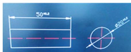
**Figure 1.** Workpiece Dimensions
