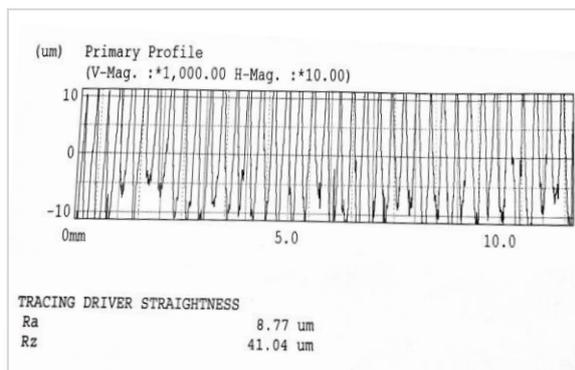
**Figure 14.** Roughest surface roughness graph.
