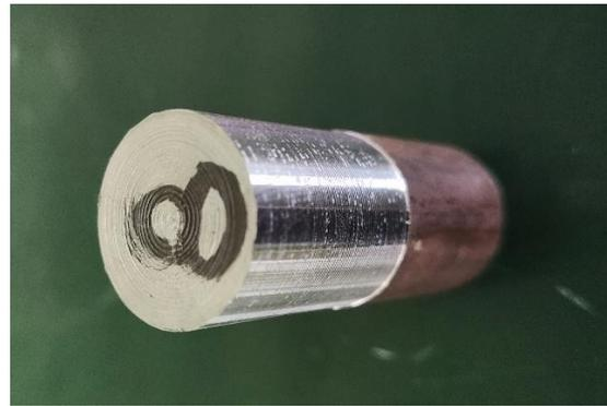
**Figure 15.** Workpiece after processing under roughest surface roughness conditions.
