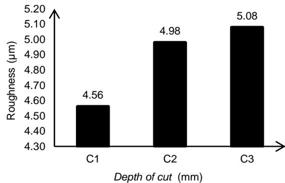
**Figure 11.** Response to surface roughness level depth of cut
