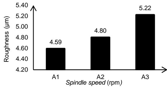
**Figure 9.** Response to surface roughness level spindle speed
