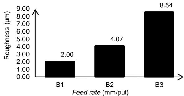
**Figure 10.** Response to surface roughness level feed rate
