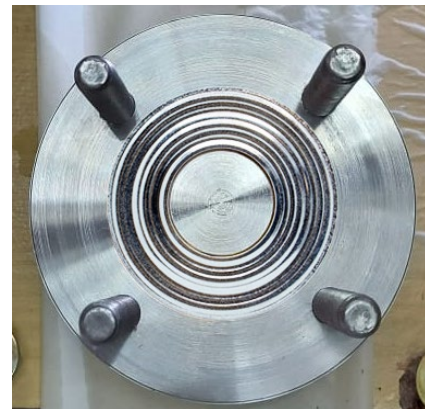
Figure 5. Gaskets inside flange
