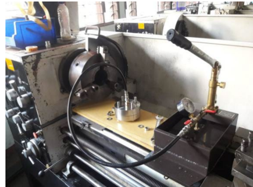
Figure 4. Leakage test equipment
