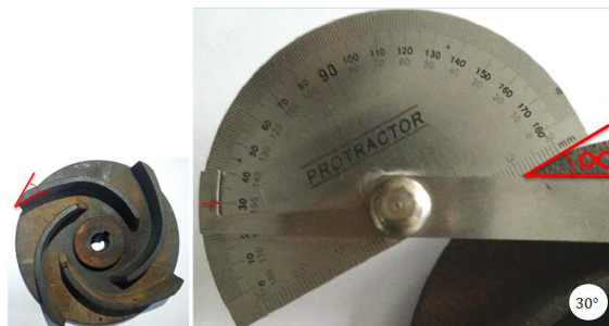
Figure 4. Impeller tip angle \alpha = 30^{\circ}
