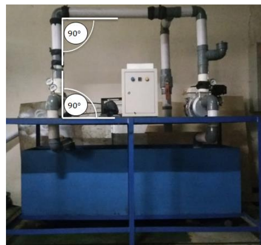
Figure 1. Entry angle Pump As Turbines (PATs) \alpha = 90^\circ
