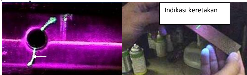
Gambar 1. Liquid Penetrant Test
