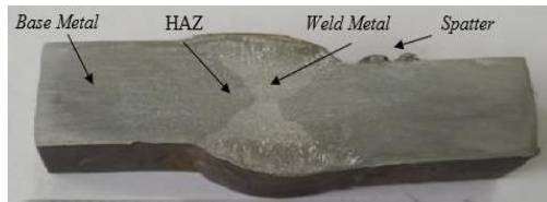
Figure 7. Macrostructure NNA sample [18]
