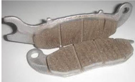
Gambar 4. Kanvas rem berbahan baku *Asbestos*<sub>[2]</sub>
