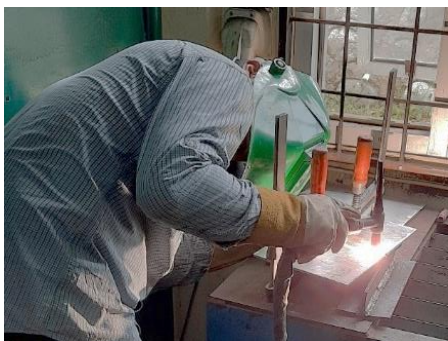
Figure 1. Aluminum welding process using TIG welding with 1G position
