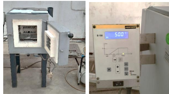
Figure 2. Solution heat treatment process with holding time variations of 1, 2, 3 hours
