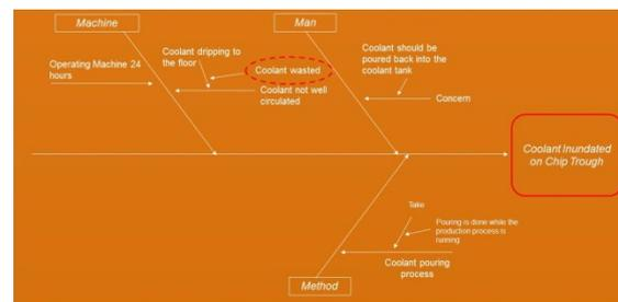
**Figure 4.** Fishbone Diagram
